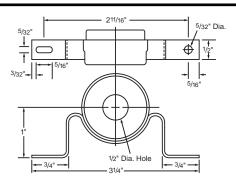
Part G-4362 **Connector Cap** Assembly (with strap) Material: Copper Cap, Beryllium Copper, Finger Stock and Strap
